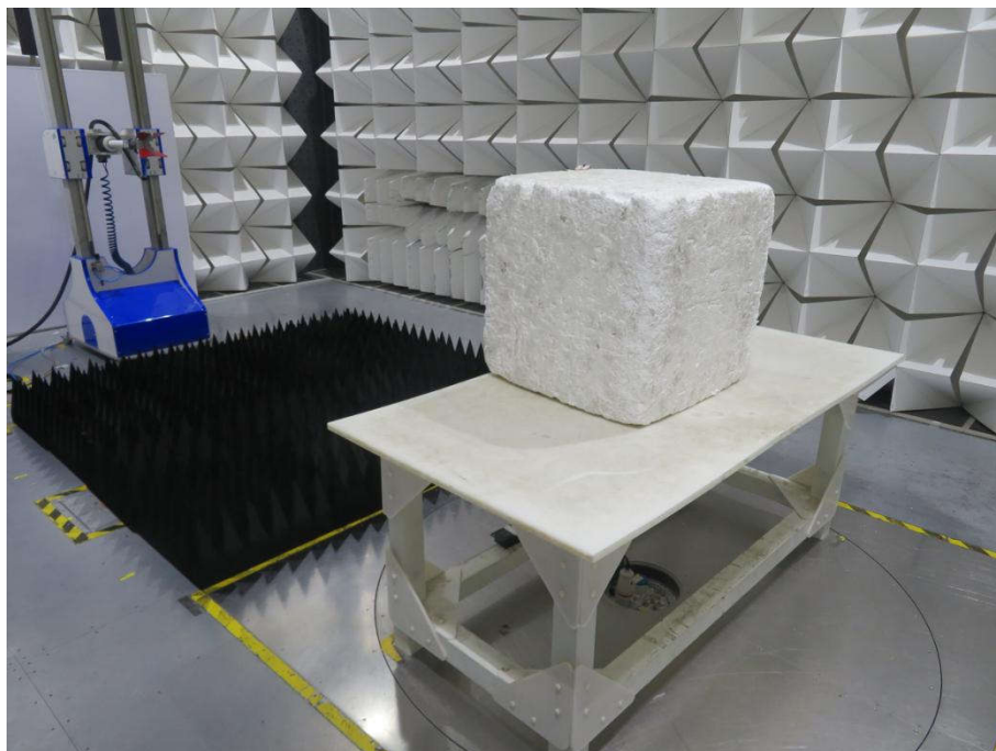
Radiated spurious emission Test Setup-2(Above 1GHz)
