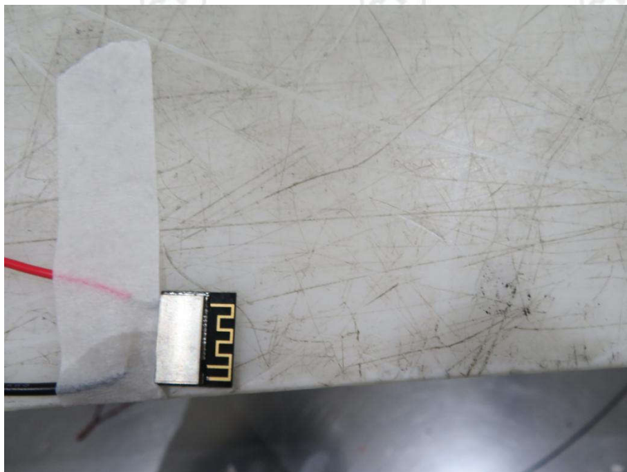
Radiated spurious emission Test Setup for close-up
