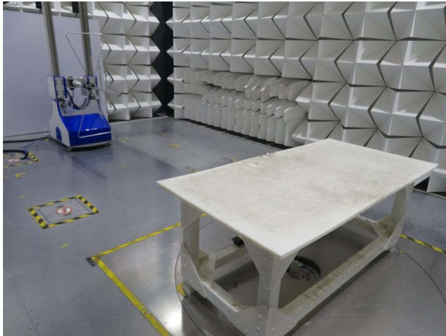
Radiated spurious emission Test Setup-1(30MHz-1GHz)
