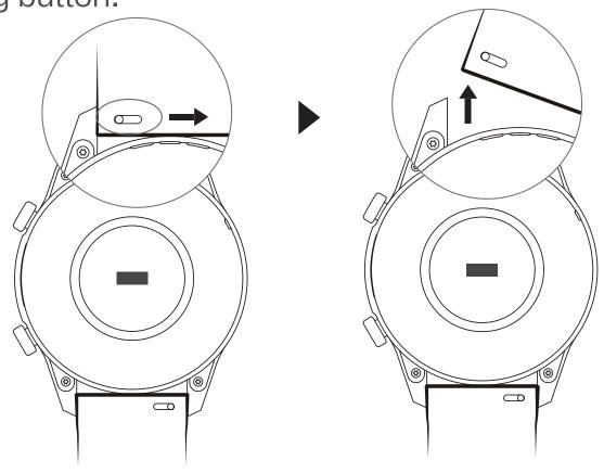
Using the reverse operation, you can install a new strap.
