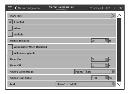
Start Test: The alarm can be tested using this button. This test will only announce the chosen alarm. It will activate the buzzer if the alarm is audible and will activate any output relays associated with this alarm. The test will not activate other common alarms or other components. To stop the testing, press the "Stop Test" button.
