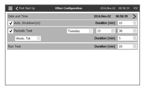
Go back to the controller start-up page and press the "Other Configuration" button. Enter the time and date. Select the "Automatic shutdown" and the duration the pump will keep running after the automatic stop if an automatic stop is desired. Select the frequency at which the periodic test will occur, the day of the week, the hour and the duration of the test. Also, enter the duration of the Manual Run Test.
