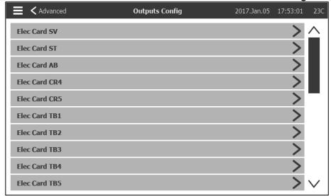
This page is used to see the logic of the signals that will activate the Outputs on the IO board and to test those Outputs. The TB6 output can also be configured from this page.
