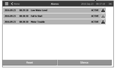
This page displays the list of currently active and occurred alarms. Alarms with adjustable parameters can be set in the Config > Advanced > Alarms pages (see section 6).
