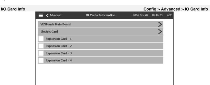
This page is used to visualize the ViZitouch and the IO Card registers by pressing on the blue arrows on the right of the screen. Expansion Cards can also be installed via this page.
