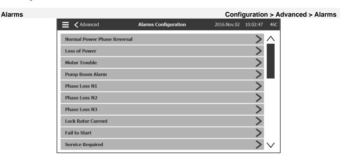
Most alarms are not configurable in the field, but some are with the appropriate password level. If it's configurable, the checkboxes will be in white. Otherwise the checkboxes will be grey. Also, the two last fields: Value Usage and Analog Value are not always visible.
