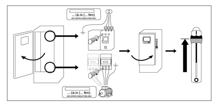
Connect the input power and the motor on their respective terminals. Secure with the appropriate torque as indicated on the torque label and verify all connections. Secure the door in closed position then put the circuit breaker disconnecting means in ON position. Verify the readings on the controller main screen.
