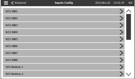
This page is for vizualisation purpose only. It allow the user to verify which signal is mapped on which controller's input.
