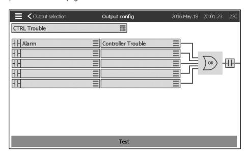
The first box from the top is used to change the name of the Output. For the output's logic, a combination of 5 digital inputs can be selected. Each input can be an alarm or a signal from a list and can be inverted by pressing the
