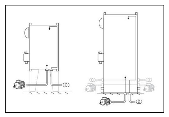
Make sure to drill holes for the motor and power connections and run the cables inside the panel, all in accordance with the specifications in order to minimize interference with other equipment.
