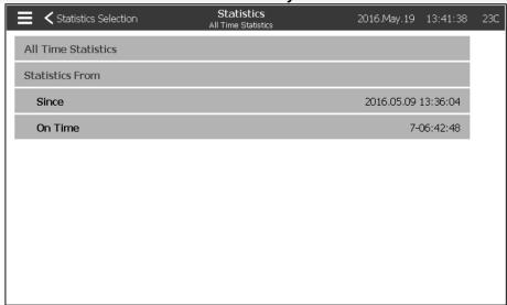
The "All Time Statistics" contains two parameters: The date the controller has been powered for the first time and the amount of time it's been ON for.
