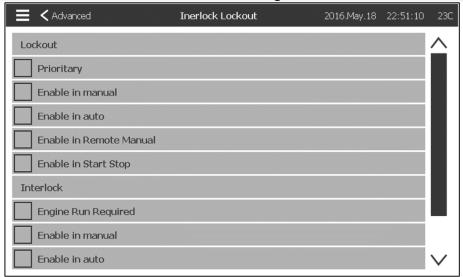
This page is used to configure the Lockout output and the Interlock input parameters. To be active those options need to be assigned to an Input or an Output on the IO board.
