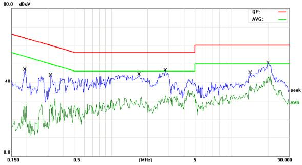
Site Chamber #2 Limit: FCC Part\_15B Class B Conduction(QP) Phase: Power: **L1** AC 120V/60Hz Temperature:
