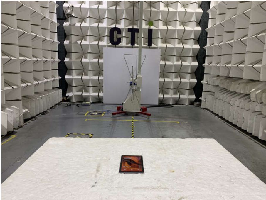
Radiated spurious emission Test Setup-1(Below 1GHz)
