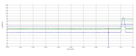
Suspected List Factor Reading Level Limit Freq. Margin NO [dB] Result Polarity Remark [MHz] [dBµV] [dBµV/m] [dBµV/m] [dB] 2390 37.56 43.33 74.00 30.67 **PASS** PΚ 5.77 Horizontal 2 2390 24.76 23.47 **PASS** 5.77 30.53 54.00 Horizontal ΑV
