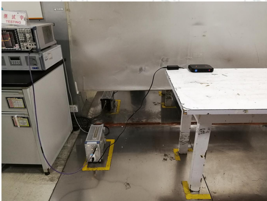
Conducted Emissions Test Setup
