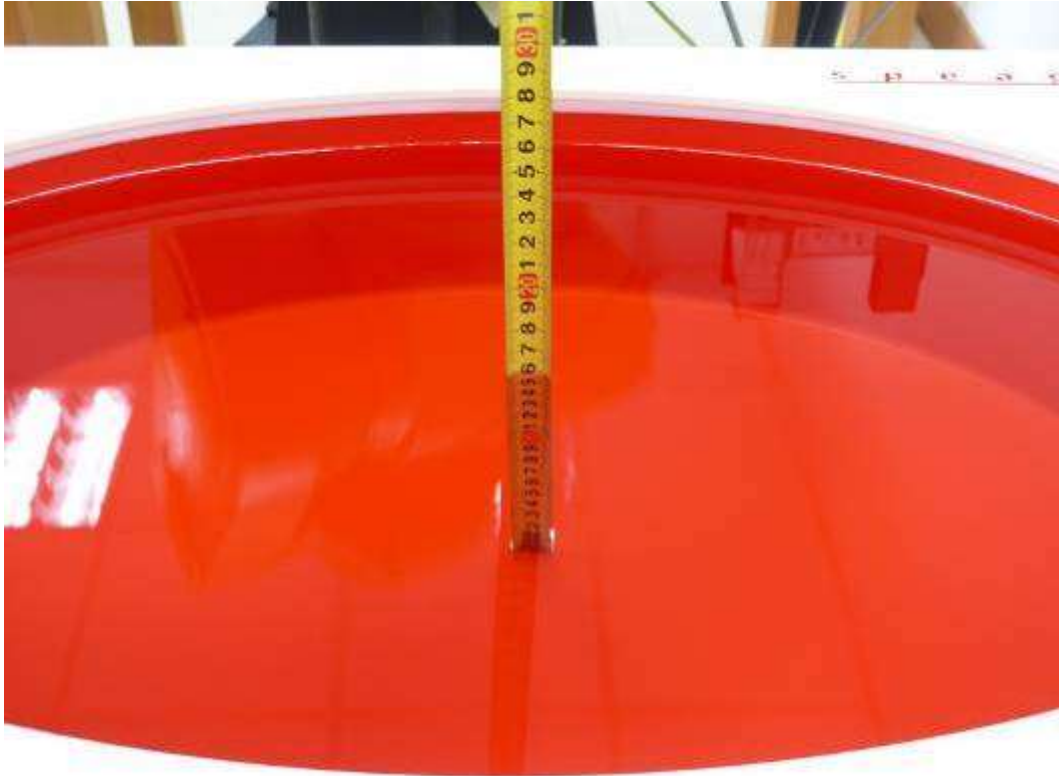
Picture 3: Liquid depth in the flat Phantom
