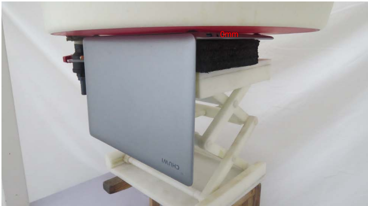
Picture 1: Back Side, the distance from handset to the bottom of the Phantom is 0mm
