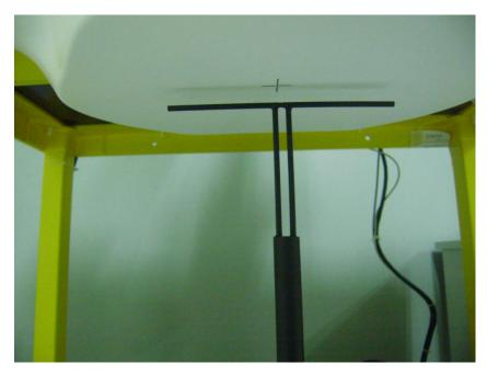
**Setup Photo of Dipole Antenna**
