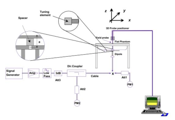
**System Verification Setup Block Diagram**
