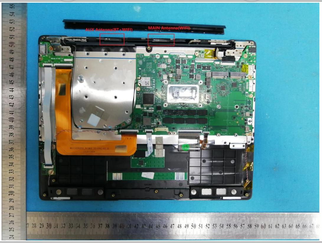
The antenna is FPC antenna. The best case gain of the antenna is 2.81dBi.
