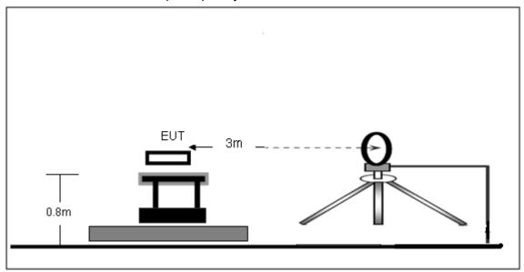
(B) Radiated Emission Test-Up Frequency 30MHz~1GHz
