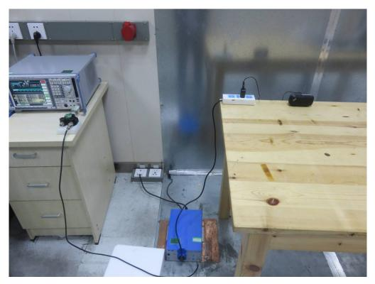
FCC RADIATED EMISSION TEST SETUP
