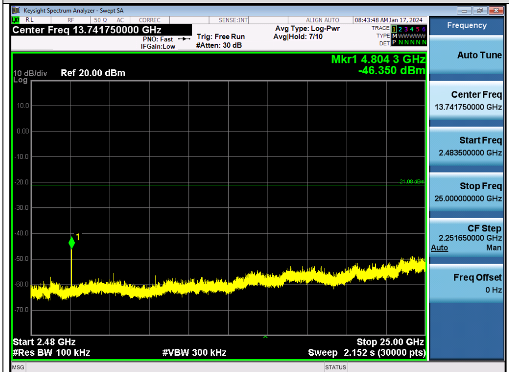
Test_Graph_EDR_ANT1_2402_2Mbps_Higher Band Emissions
