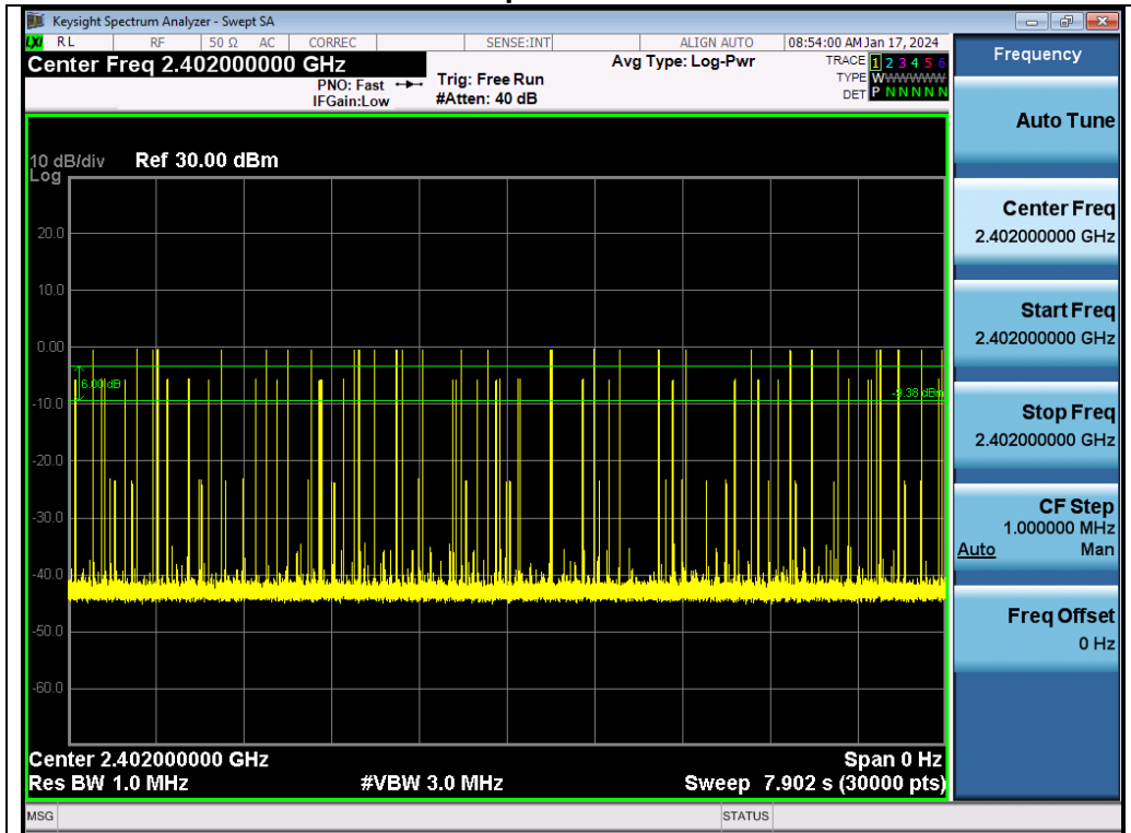
Test_Graph_EDR_HOP_ANT1_NA_2Mbps_2402_Number of Burst
