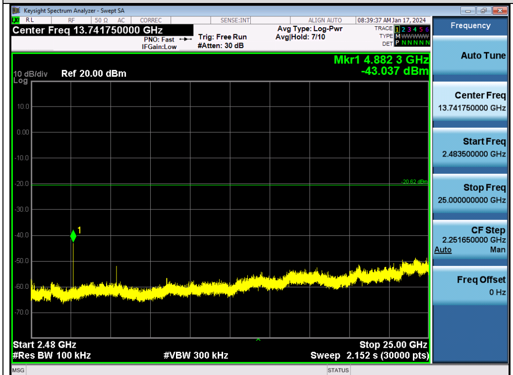
Test_Graph_BR_ANT1_2441_1Mbps_Higher Band Emissions
