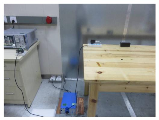
FCC RADIATED EMISSION TEST SETUP
