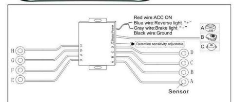
The rear sensors A,B,C,D should be installed from left to right.
