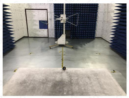
RADIATED EMISSION TEST SETUP ABOVE 1GHz
