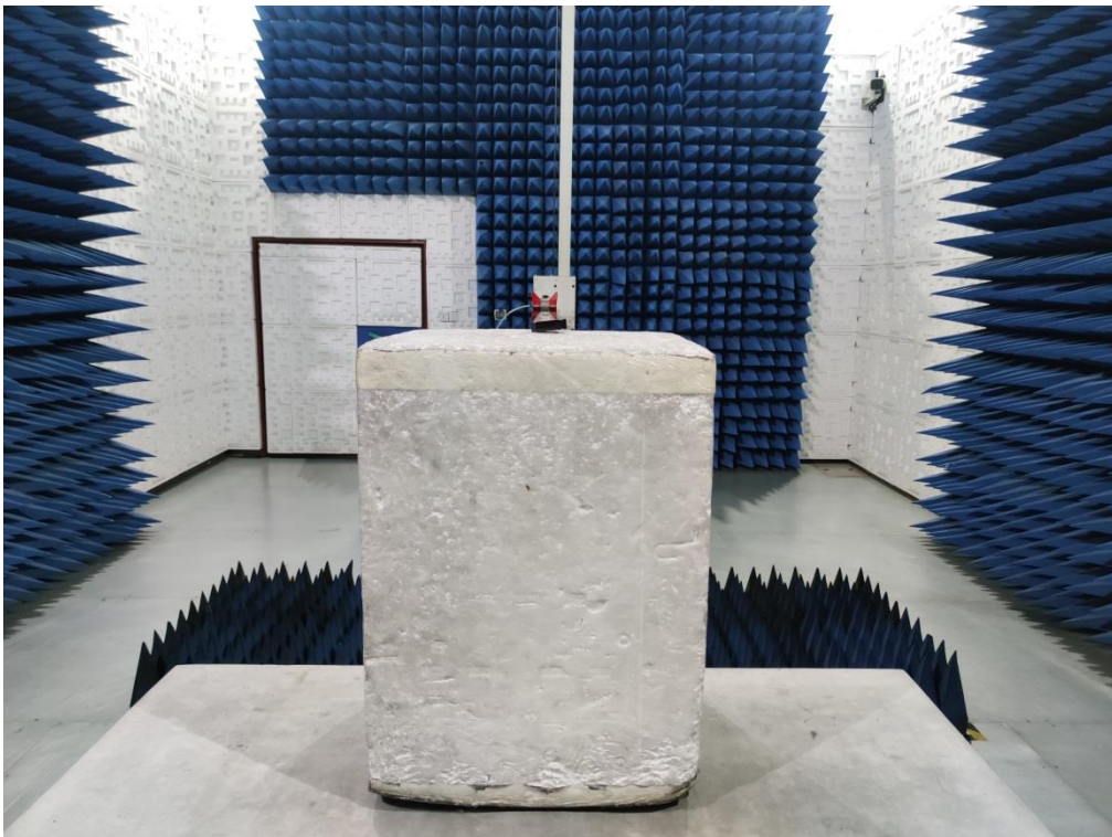
RADIATED EMISSION TEST SETUP ABOVE 1GHZ
