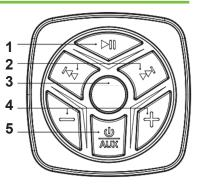
**5 Power/Aux button -** Pressing this button once will turn the IBBTR19 on or off. A quick double press of this button will switch the audio source to the auxiliary input. Double press this button again to switch back to wireless mode.
