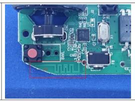
The antenna is PCB antenna.
