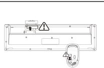
Open the battery covers and insert a AAA battery in the keyboard and a AA battery in the mouse.
