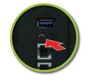
Press this button to start the procedure for setting up WPS (PBC). Press PBC button of your wireless clients within coverage area in two minutes to allow joining the wireless network.
