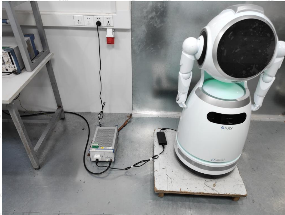
Photo of Conducted Emission Test
