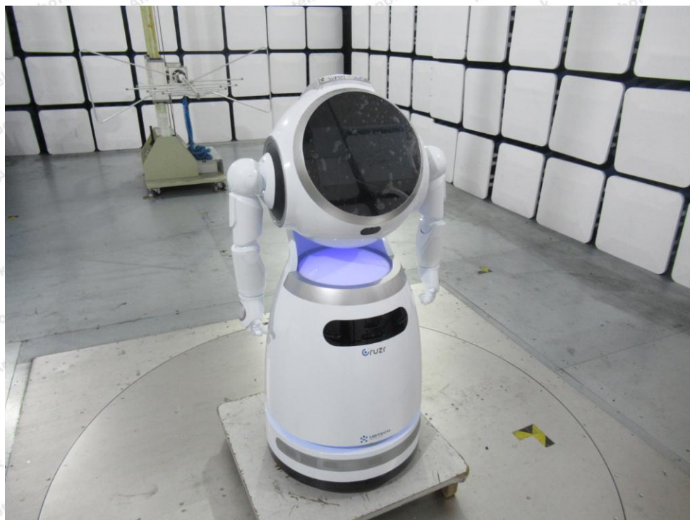
Photo of Radiation Emission Test
