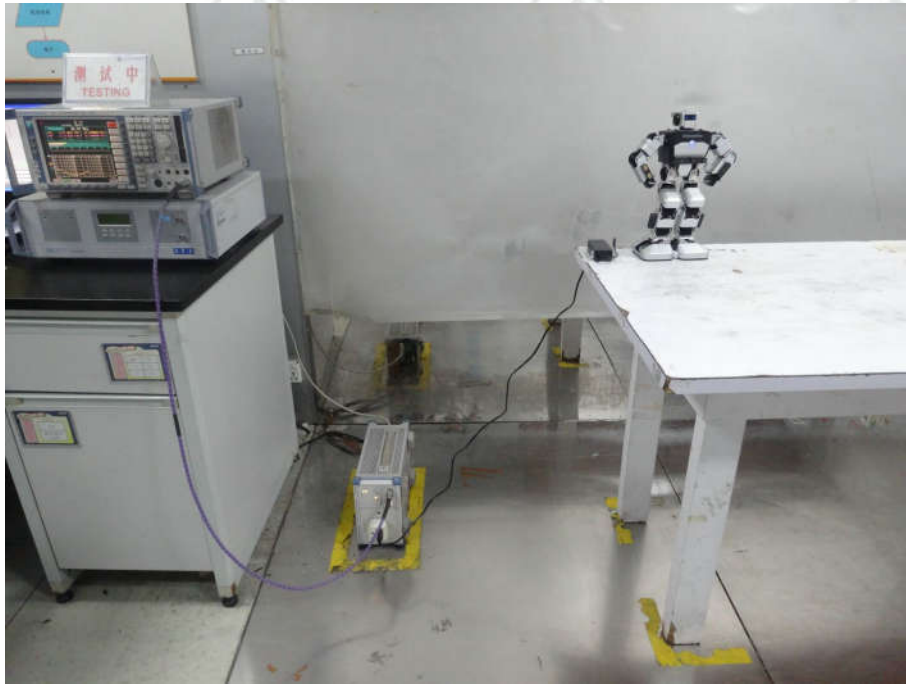
Conducted Emissions Test Setup
