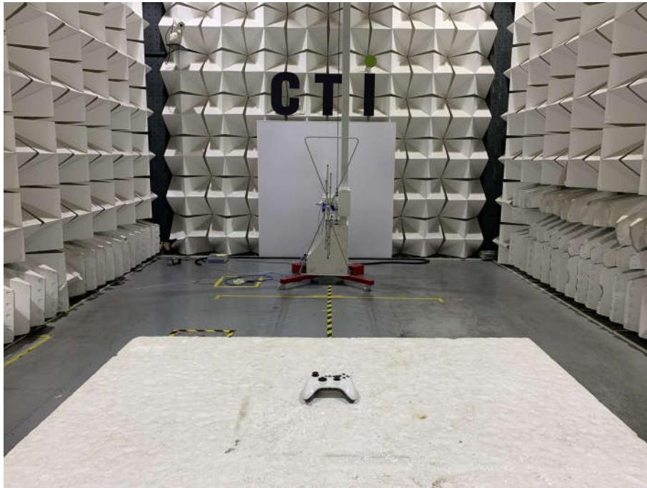
Radiated spurious emission Test Setup-1(Below 1GHz)
