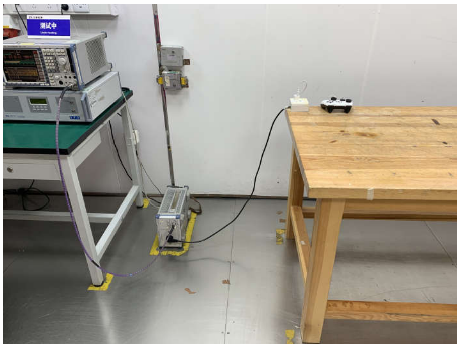
Conducted Emissions Test Setup
