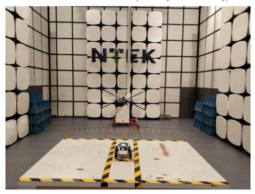
Radiated Measurement Photos (Power by alkaline battery)
