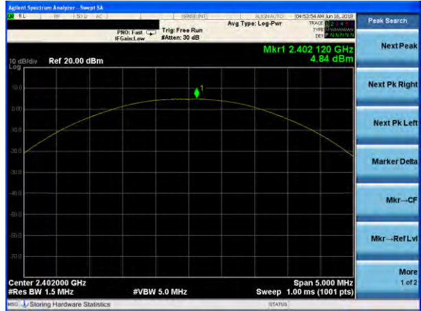
Peak output Power plot on channel 39 (2Mbps)
