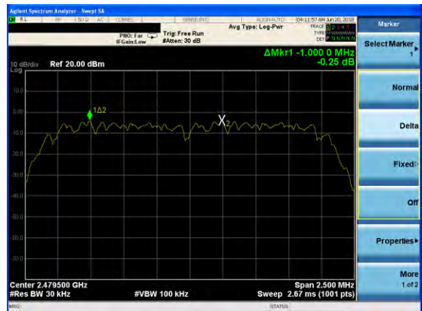
(2Mbps) Channel Separation plot on channel 77-78
