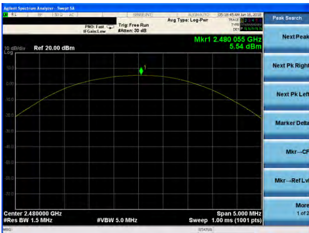
Peak output Power plot on channel 78 (3Mbps)
