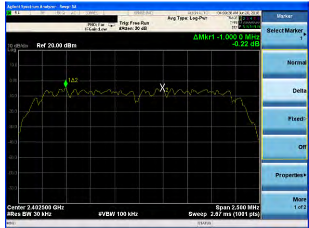
(2Mbps) Channel Separation plot on channel 39-40
