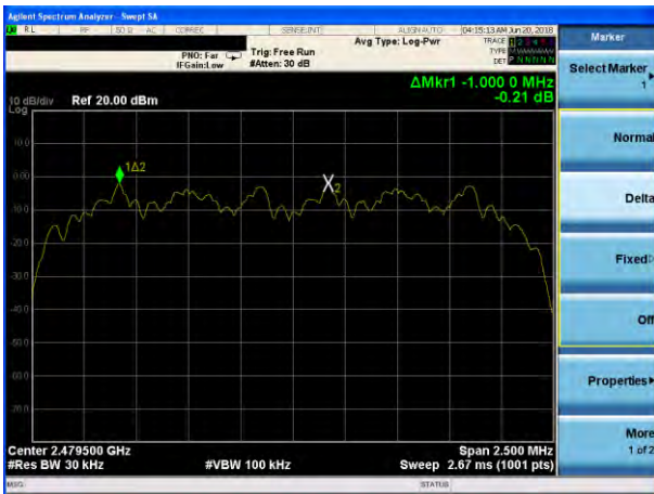
(3Mbps) Channel Separation plot on channel 77-78
