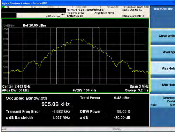
20dB Bandwidth plot on channel 39 (1Mbps)
