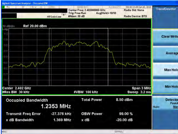
20dB Bandwidth plot on channel 39 (3Mbps)
