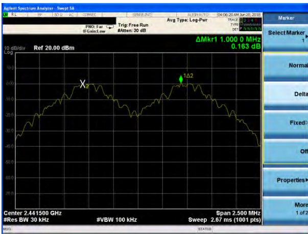
(1Mbps) Channel Separation plot on channel 77-78
