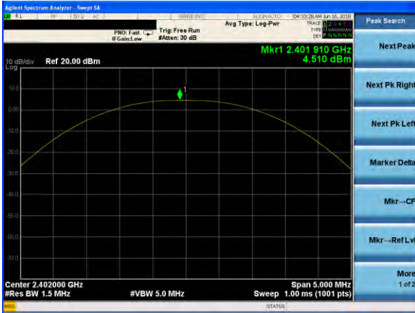
Peak output Power plot on channel 39 (1Mbps)
