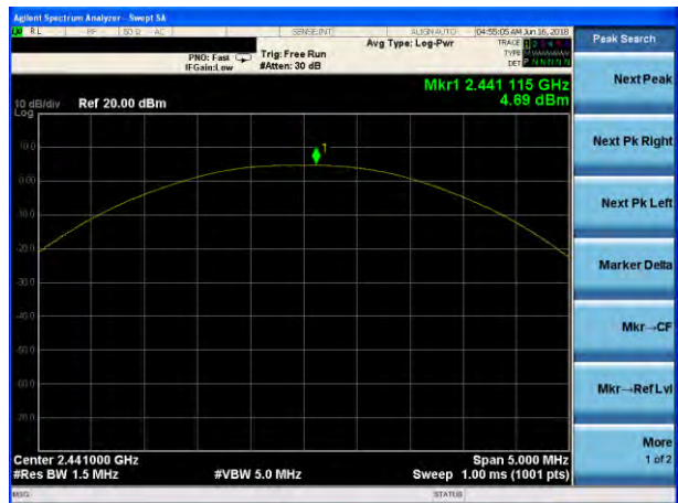
Peak output Power plot on channel 39 (2Mbps)
