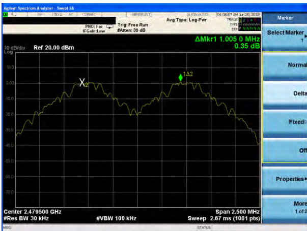
(1Mbps) Channel Separation plot on channel 77-78
