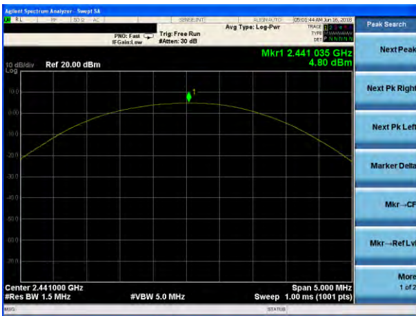
Peak output Power plot on channel 39 (3Mbps)
