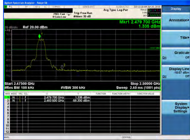
8-DPSK: Band Edge-High Channel
