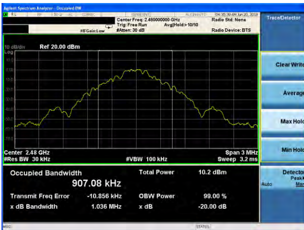
20dB Bandwidth plot on channel 78 (1Mbps)
