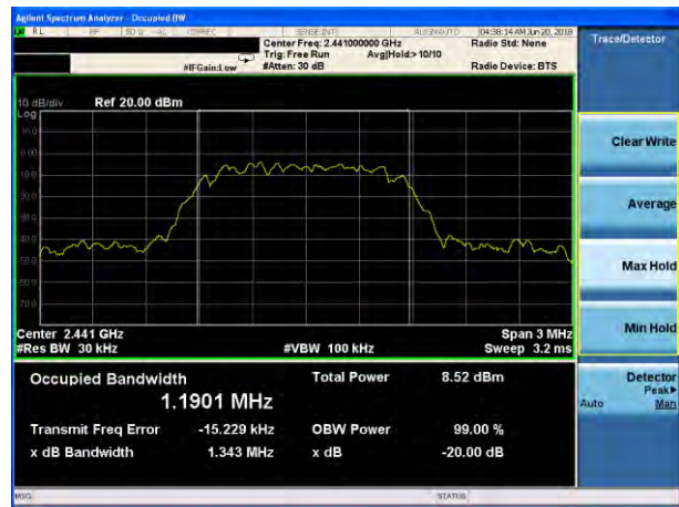
20dB Bandwidth plot on channel 78 (2Mbps)
