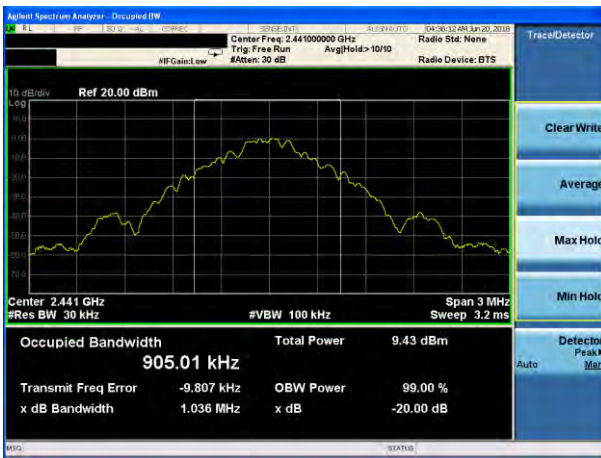
20dB Bandwidth plot on channel 78 (1Mbps)
