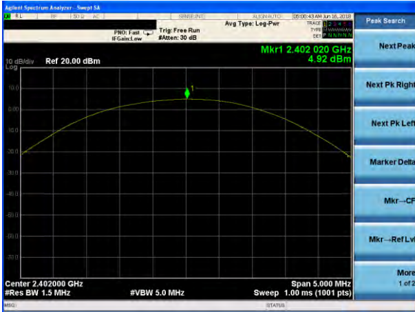
Peak output Power plot on channel 39 (3Mbps)
