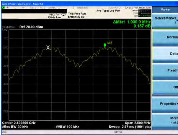
(1Mbps) Channel Separation plot on channel 39-40
