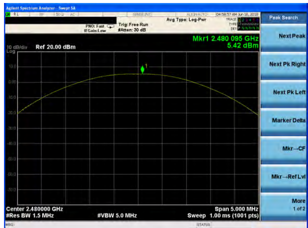
Peak output Power plot on channel 78 (2Mbps)
