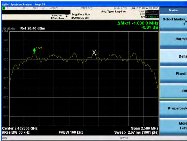
(3Mbps) Channel Separation plot on channel 39-40
