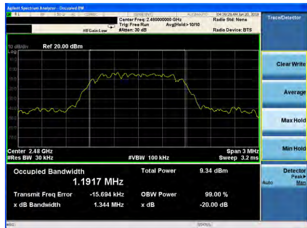
20dB Bandwidth plot on channel 78 (2Mbps)
