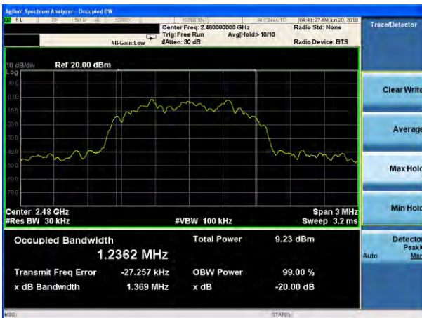
20dB Bandwidth plot on channel 78 (3Mbps)
