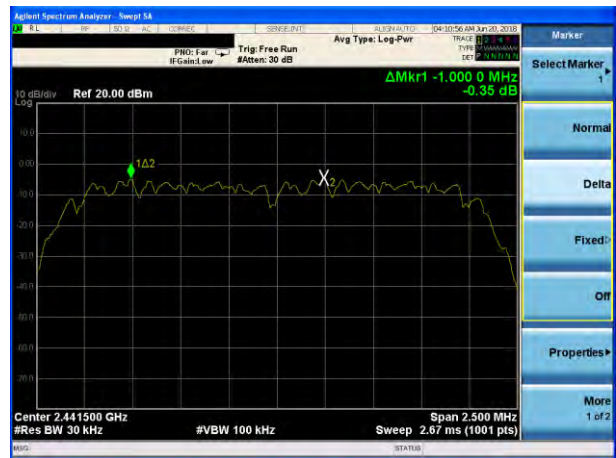
(2Mbps) Channel Separation plot on channel 77-78
