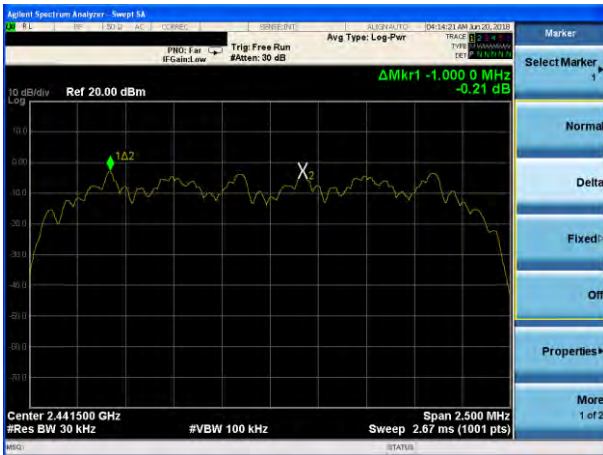
(3Mbps) Channel Separation plot on channel 39-40
