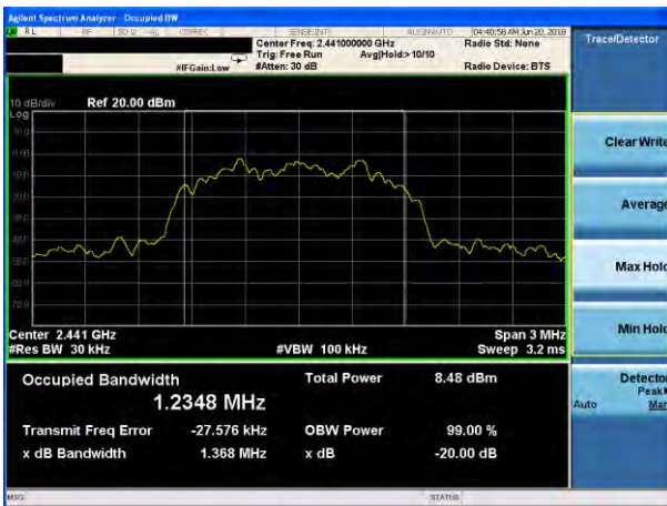
20dB Bandwidth plot on channel 39 (3Mbps)
