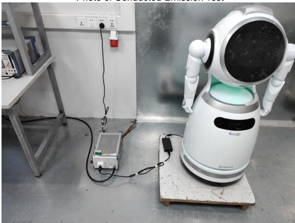
Photo of Conducted Emission Test
