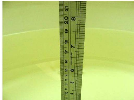
Fig 7.2 Photo of Liquid Height for Body SAR
