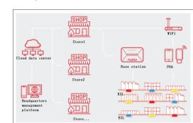
The tag is automatically managed by the server through 2.4G, which can realize different operation scenarios: display the tag IP, scan the IP through the handset or bind / unbind the app with the commodity barcode, and apply for re obtaining the price tag data from the base station
