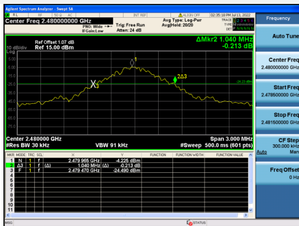
GFSK HIGH CHANNEL
