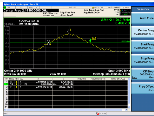
GFSK MIDDLE CHANNEL
