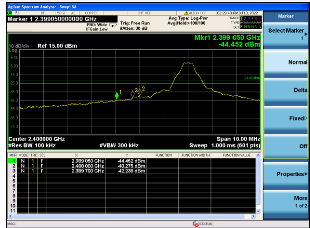
GFSK LOW CHANNEL, BAND EDGE
