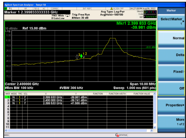
GFSK LOW CHANNEL, BAND EDGE
