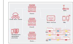
The tag is automatically managed by the server through 2.4G, which can realize different operation scenarios: display the tag IP, scan the IP through the handset or bind / unbind the app with the commodity barcode, and apply for re obtaining the price tag data from the base station.
