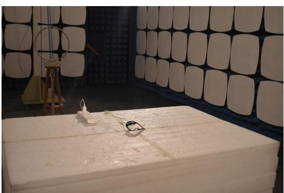
3. Radiated emission (9KHz-30MHz)
