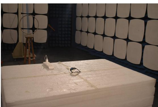
3. Radiated emission (9KHz-30MHz)
