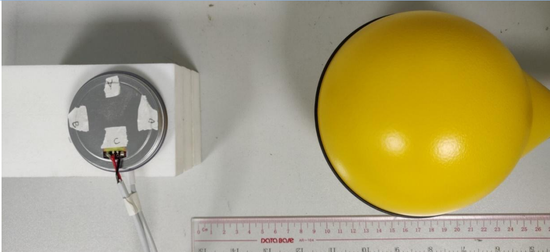
H-field Test Setup Photo of Position D(15cm)
