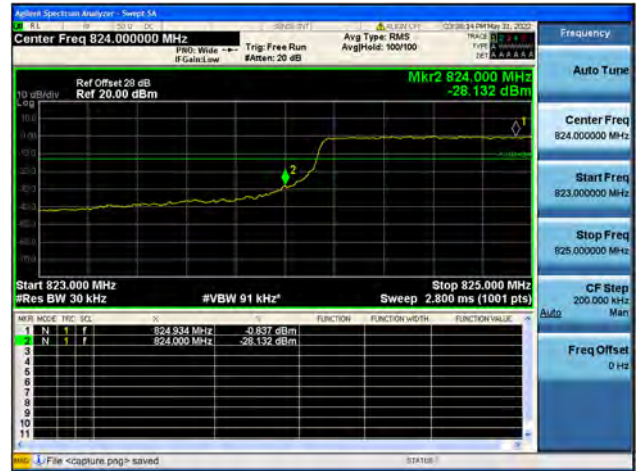
B5 / 3MHz / High CH / QPSK / FULL RB
