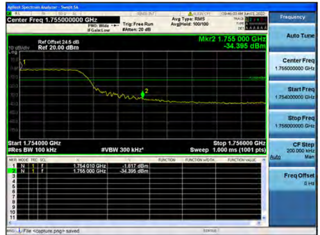
B4 / 10MHz / High CH / QPSK / FULL RB
