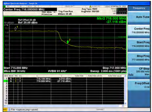
B12 / 1.4MHz / High CH / QPSK / FULL RB
