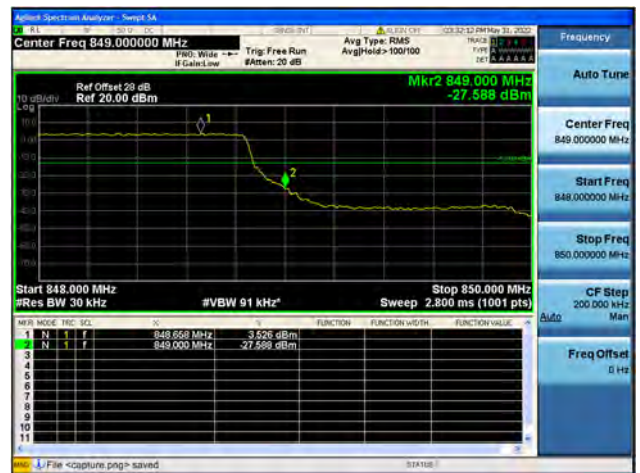
Band26 / 1.4MHz / High CH / QPSK / FULL RB
