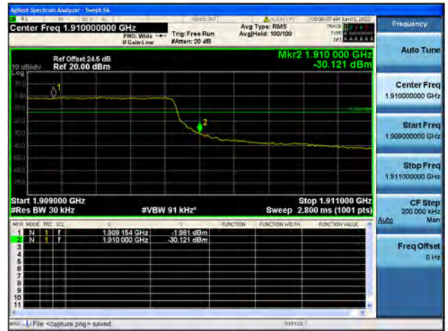
B2 / 3MHz / High CH / QPSK / FULL RB
