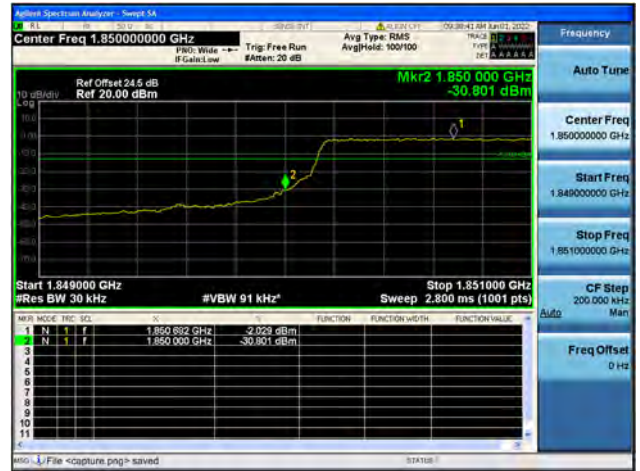
B2 / 3MHz / High CH / QPSK / FULL RB
