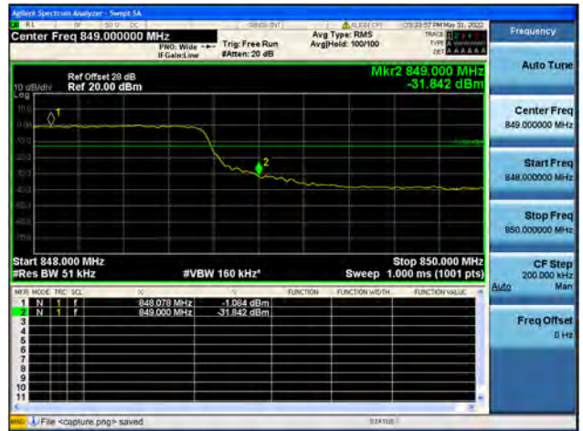
Band26 / 5MHz / High CH / QPSK / FULL RB
