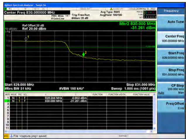
B18Part22 / 5MHz / High CH / QPSK / FULL RB
