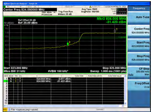
B18Part22 / 5MHz / High CH / QPSK / FULL RB
