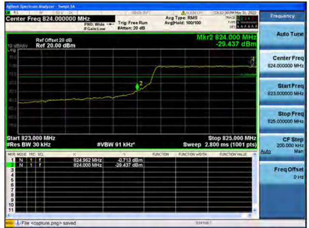
Band26 / 3MHz / High CH / QPSK / FULL RB
