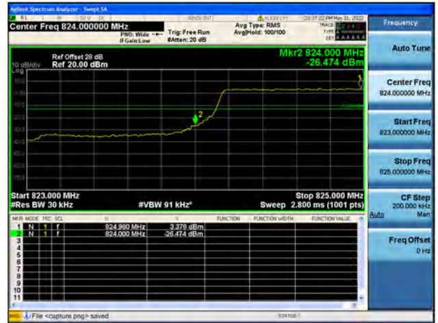
B5 / 1.4MHz / High CH / QPSK / FULL RB
