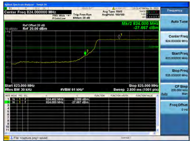
Band26 / 1.4MHz / High CH / QPSK / FULL RB
