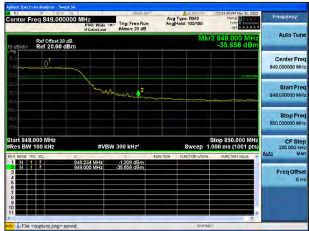
Band26 / 10MHz / High CH / QPSK / FULL RB
