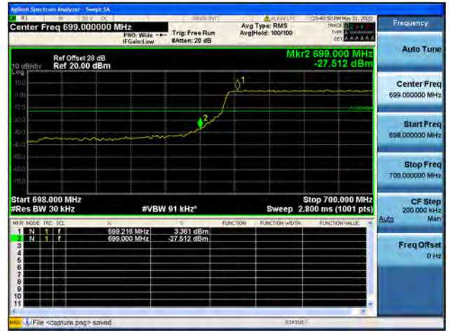
B12 / 1.4MHz / High CH / QPSK / FULL RB
