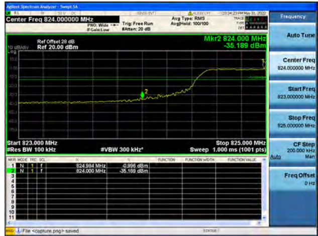
Band26 / 10MHz / High CH / QPSK / FULL RB
