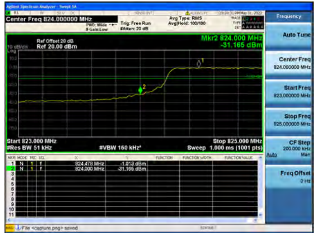
Band26 / 5MHz / High CH / QPSK / FULL RB
