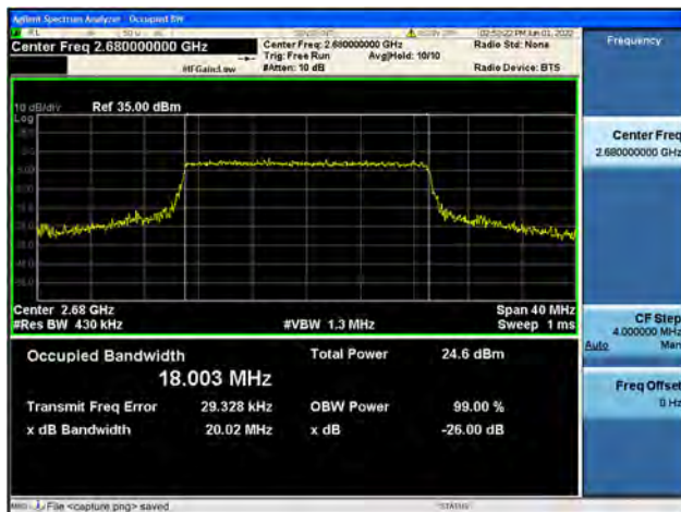
B41 / 20MHz / 16QAM/ High CH
