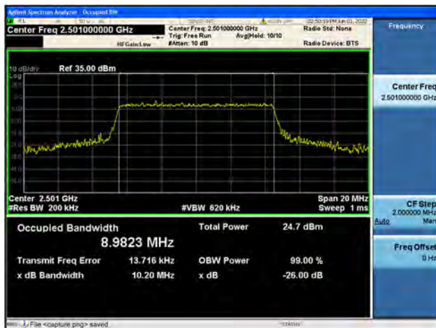
B41 / 10MHz / 16QAM/ Low CH
