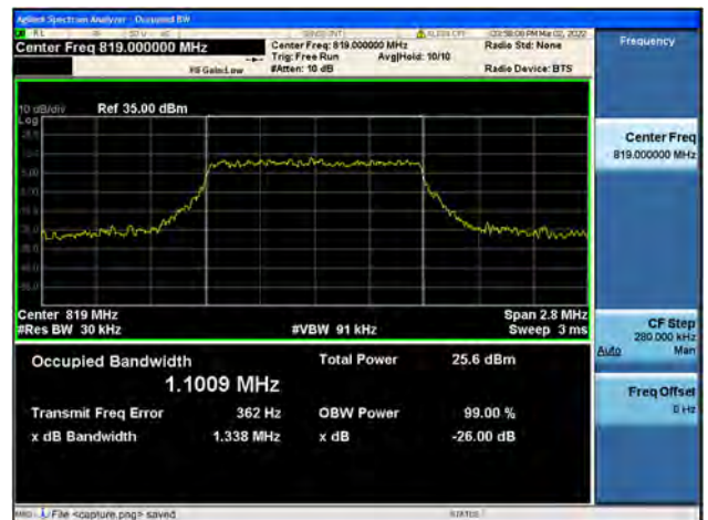
Band26 / 1.4MHz / Mid CH / 64QAM
