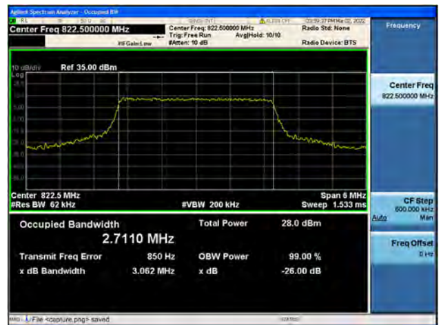
Band26 / 3MHz / High CH / 64QAM
