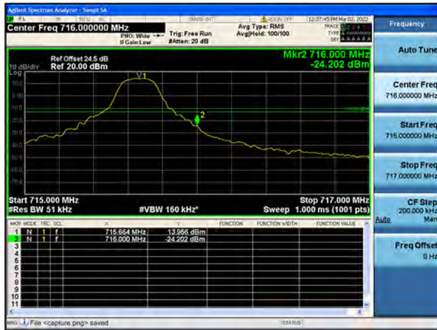
Band12 / 5MHz / High CH / QPSK / 1 RB
