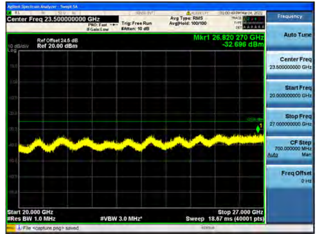
Band41 / 15MHz / Mid CH / 16QAM
