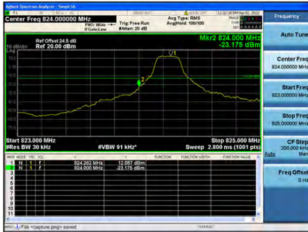
Band5 / 3MHz / High CH / QPSK / 1 RB
