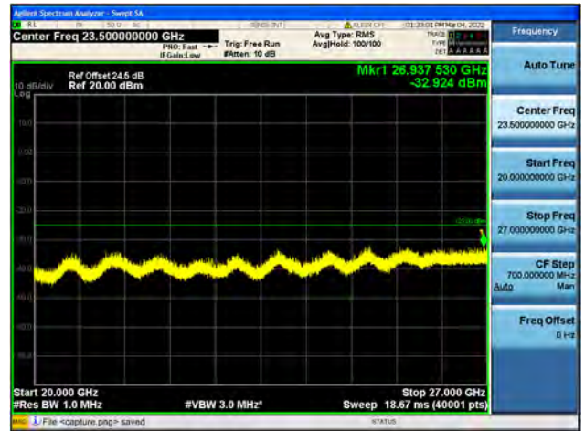
Band41 / 15MHz / Mid CH / 64QAM
