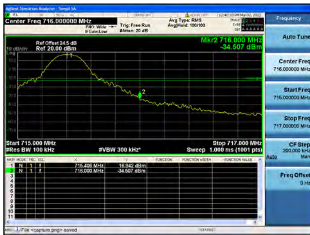
Band17 / 10MHz / High CH / QPSK / 1 RB
