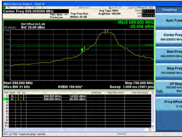
Band12 / 5MHz / High CH / QPSK / 1 RB
