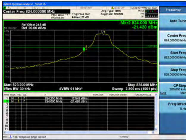
Band5 / 1.4MHz / High CH / QPSK / 1 RB
