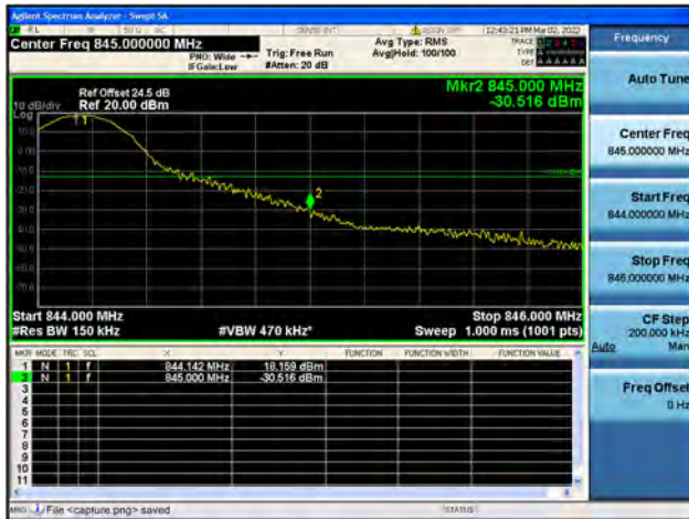
Band19 / 15MHz / High CH / QPSK / 1 RB
