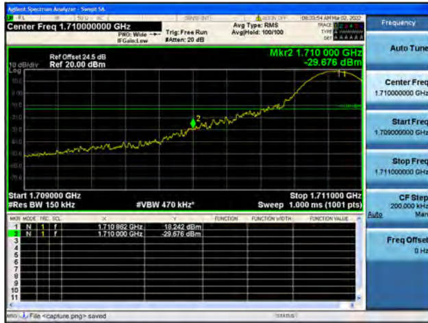
Band4 / 15MHz / High CH / QPSK / 1 RB
