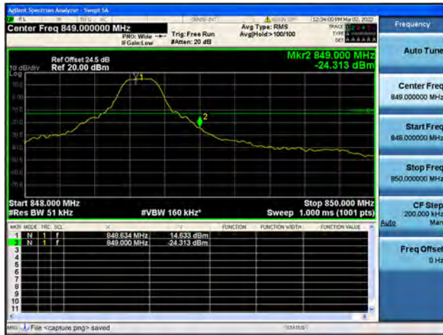
Band5 / 5MHz / High CH / QPSK / 1 RB
