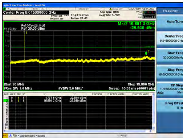
Band66 / 3MHz / High CH / 16QAM
