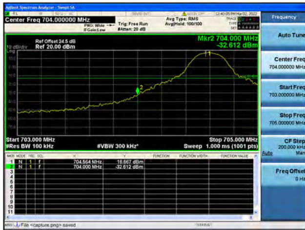
Band17 / 10MHz / High CH / QPSK / 1 RB
