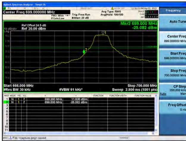
Band12 / 3MHz / High CH / QPSK / 1 RB
