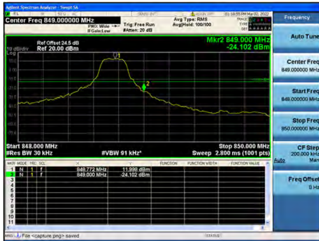
Band26 / 3MHz / High CH / QPSK / 1 RB
