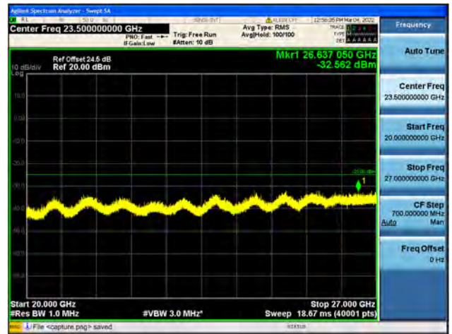
Band41 / 10MHz / High CH / 16QAM
