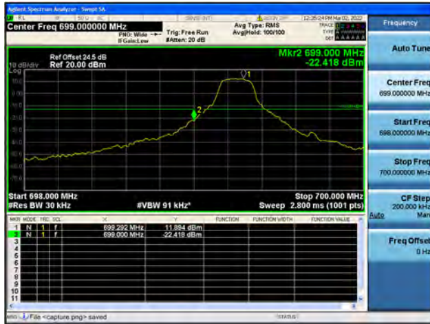
Band12 / 1.4MHz / High CH / QPSK / 1 RB
