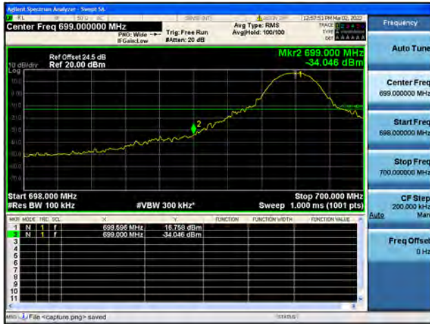
Band12 / 10MHz / High CH / QPSK / 1 RB
