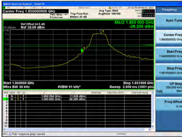
Band2 / 3MHz / High CH / QPSK / 1 RB
