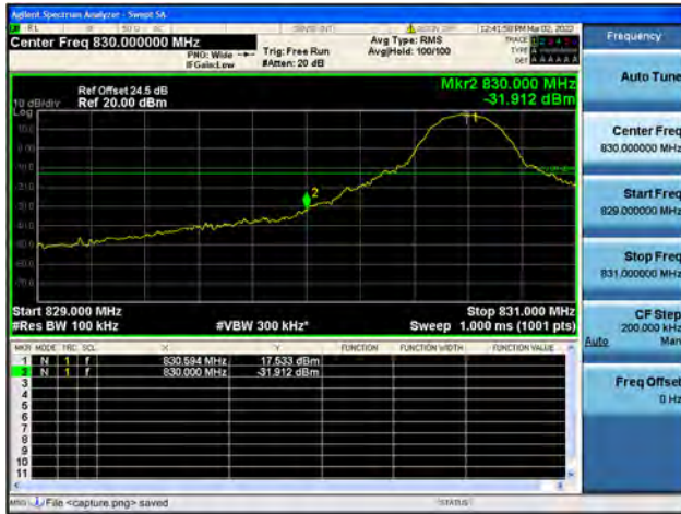
Band19 / 10MHz / High CH / QPSK / 1 RB
