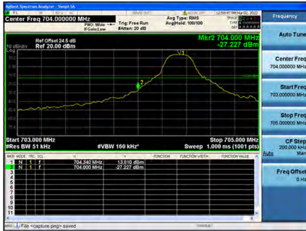
Band17 / 5MHz / High CH / QPSK / 1 RB
