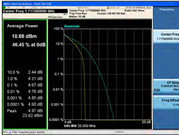
Band66 / 15MHz / Low CH / 64QAM
