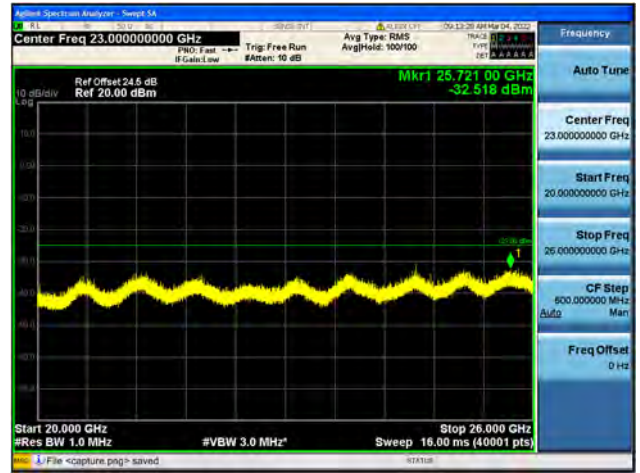
Band7 / 10MHz / High CH / 16QAM
