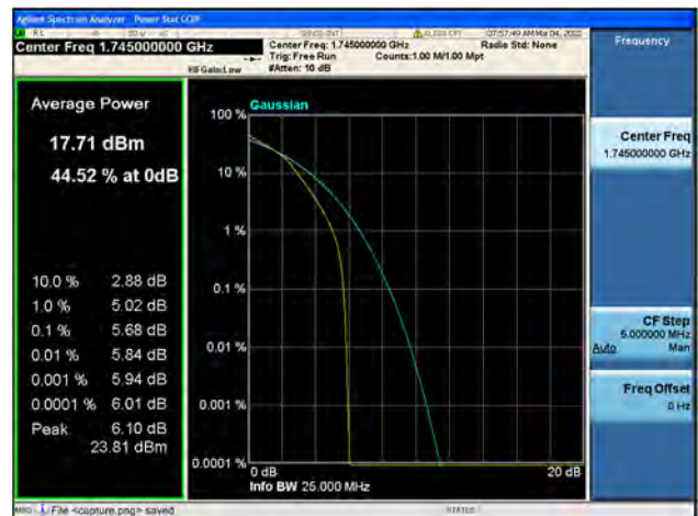
Band66 / 15MHz / Mid CH / 64QAM
