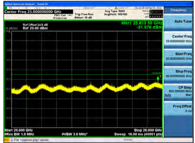
Band7 / 15MHz / High CH / 16QAM
