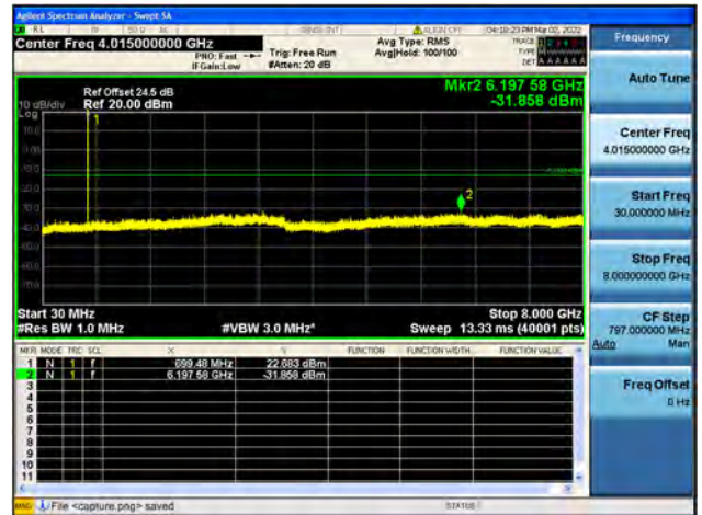
Band12 / 3MHz / Low CH / 64QAM
