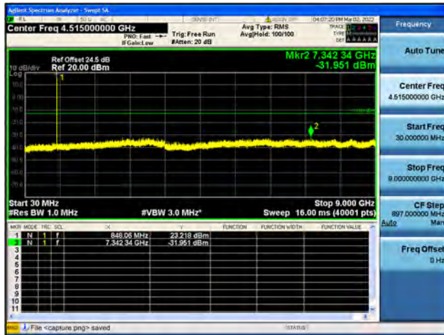
Band5 / 3MHz / Low CH / 16QAM
