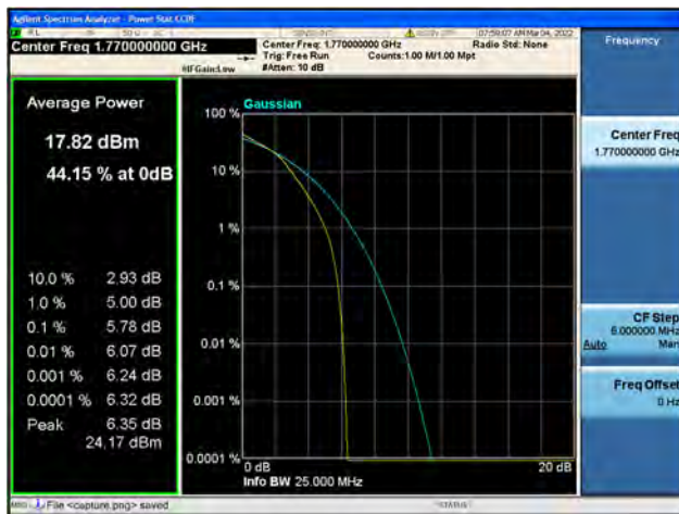
Band66 / 20MHz / High CH / 16QAM
