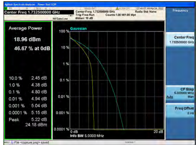
Band4 / 5MHz / Mid CH / 64QAM
