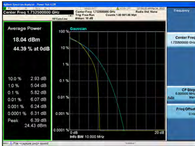
Band4 / 10MHz / High CH / 16QAM
