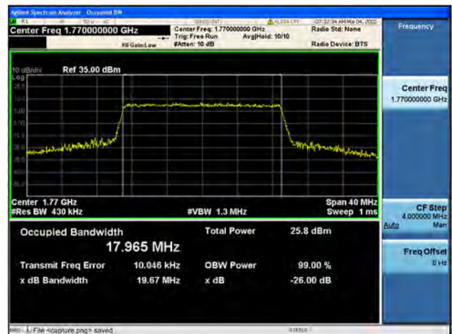
Band66 / 20MHz / High CH / 64QAM
