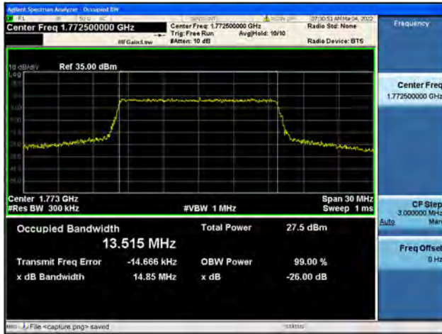
Band66 / 15MHz / High CH / 64QAM
