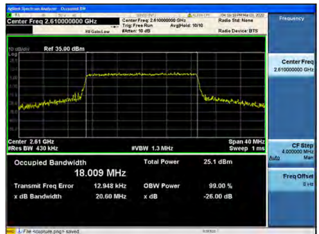
Band38 / 20MHz / High CH / 64QAM
