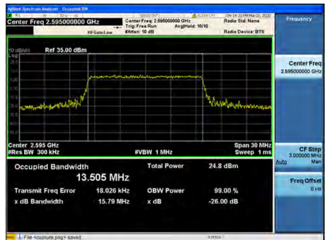
Band38 / 15MHz / Mid CH / 64QAM
