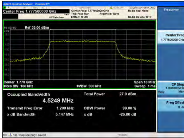
Band66 / 5MHz / High CH / 64QAM
