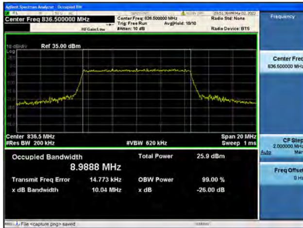
Band26 / 10MHz / High CH / 16QAM
