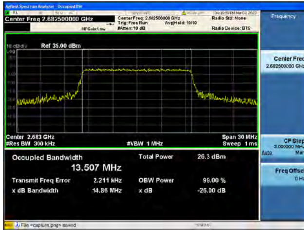
Band41 / 15MHz / High CH / 64QAM
