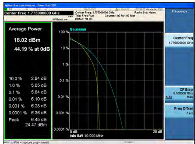
Band66 / 10MHz / High CH / 64QAM
