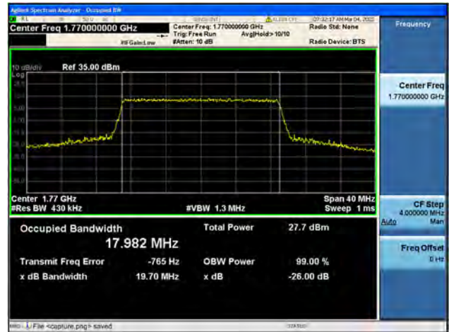
Band66 / 20MHz / High CH / 64QAM
