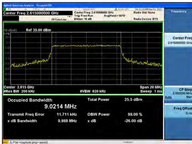
Band38 / 10MHz / High CH / 16QAM
