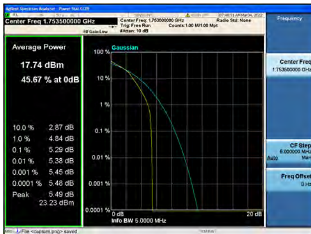
Band4 / 3MHz / High CH / 16QAM
