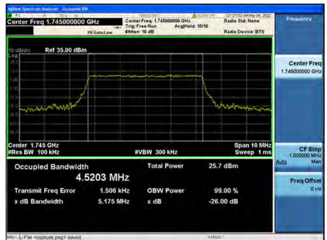
Band66 / 5MHz / Mid CH / 64QAM
