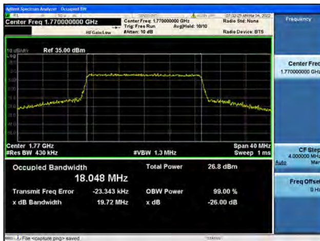
Band66 / 20MHz / High CH / 16QAM
