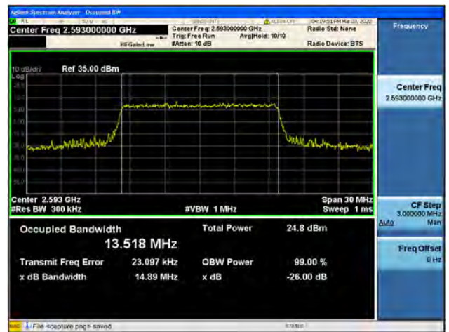
Band41 / 15MHz / Mid CH / 64QAM
