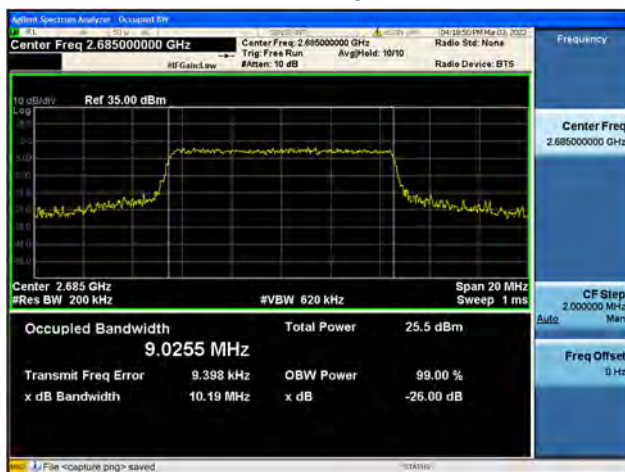
Band41 / 10MHz / High CH / 16QAM
