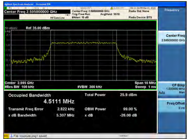
Band38 / 5MHz / Mid CH / 64QAM
