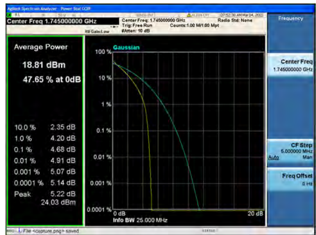
Band4 / 20MHz / High CH / 64QAM
