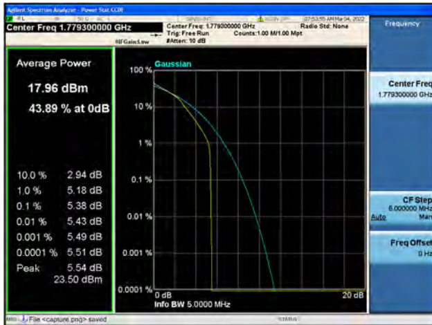
Band66 / 3MHz / Low CH / 16QAM
