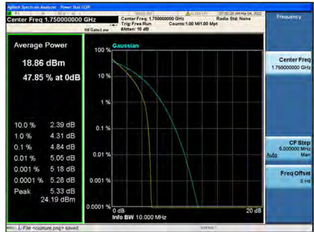
Band4 / 10MHz / High CH / 64QAM
