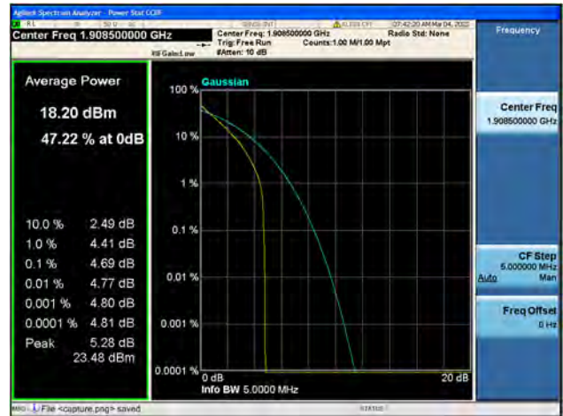
Band2 / 3MHz / High CH / 64QAM
