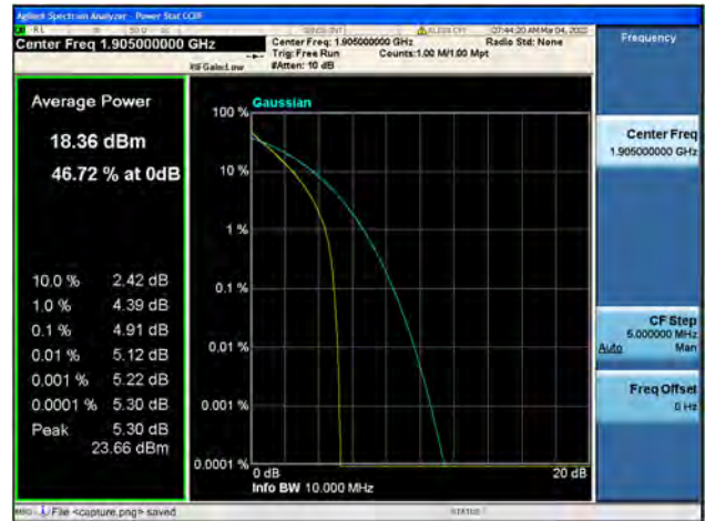
Band2 / 10MHz / High CH / 64QAM
