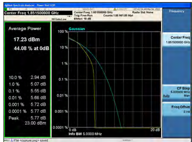
Band2 / 3MHz / Low CH / 64QAM
