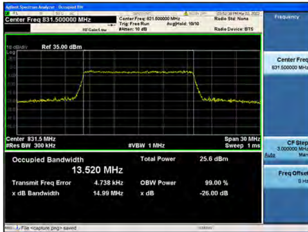
Band26 / 15MHz / Mid CH / 16QAM
