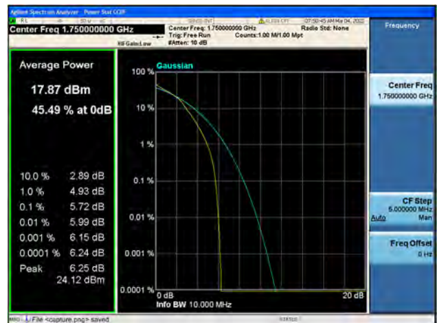
Band4 / 10MHz / High CH / 64QAM
