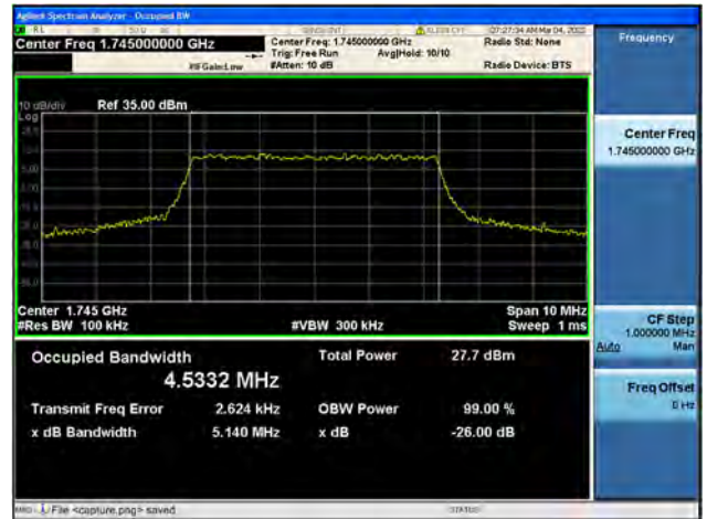
Band66 / 5MHz / Mid CH / 64QAM
