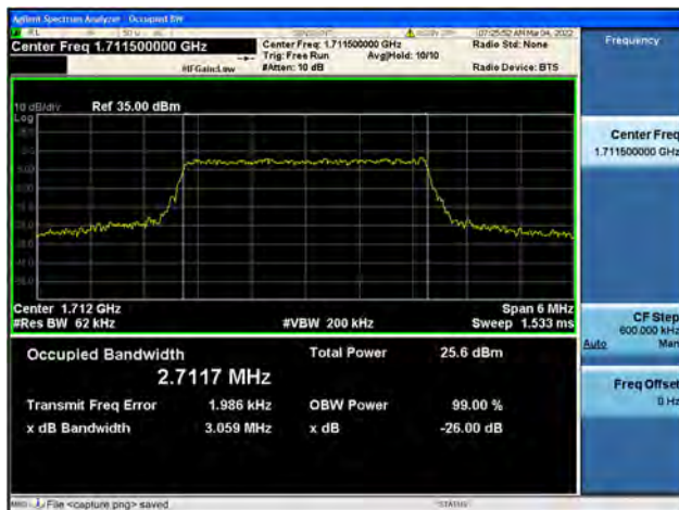
Band66 / 3MHz / Low CH / 16QAM
