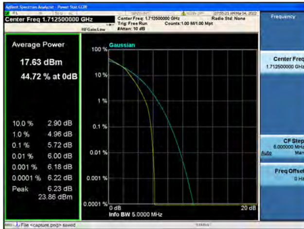
Band66 / 5MHz / Mid CH / 16QAM
