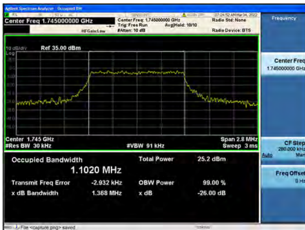
Band66 / 1.4MHz / Mid CH / 16QAM
