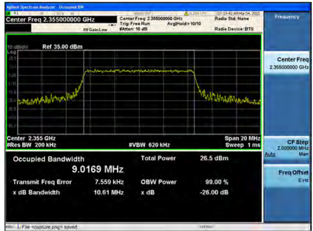
Band40/ Block B / 10MHz / Mid CH / 64QAM
