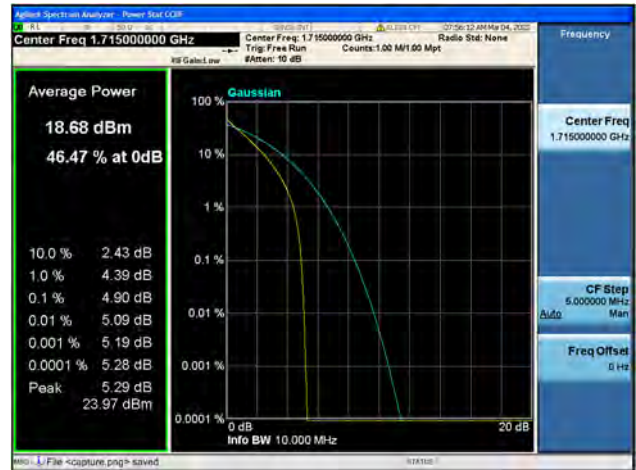
Band66 / 10MHz / Low CH / 64QAM
