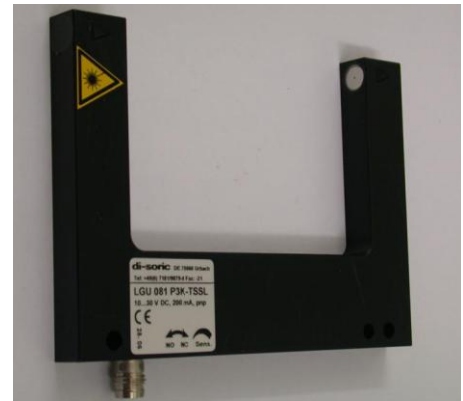
Fig. 6.7 Photo of Light Beam
