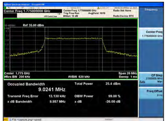
Band66 / 10MHz / High CH / 64QAM
