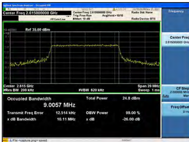
Band38 / 10MHz / High CH / 16QAM
