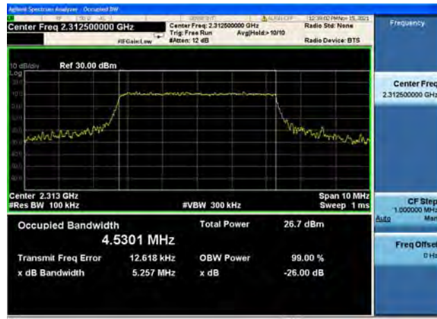
Band40/ Block A / 5MHz / High CH / 64QAM
