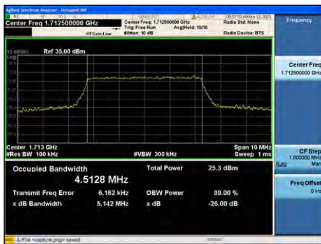
Band66 / 5MHz / Mid CH / 16QAM
