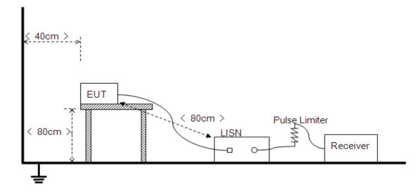
The EUT is placed on a 0.8m high insulating table, which stands on the grounded conducting floor, and keeps 0.4m away from the grounded conducting wall. The EUT is connected to the power mains through a LISN which provides  $50\Omega/50\mu$ H of coupling impedance for the measuring instrument. A Pulse Limiter is used to protect the measuring instrument. The factors of the whole test system are calibrated to correct the reading.
