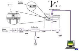
Fig 8.2 System Setup for System Evaluation
