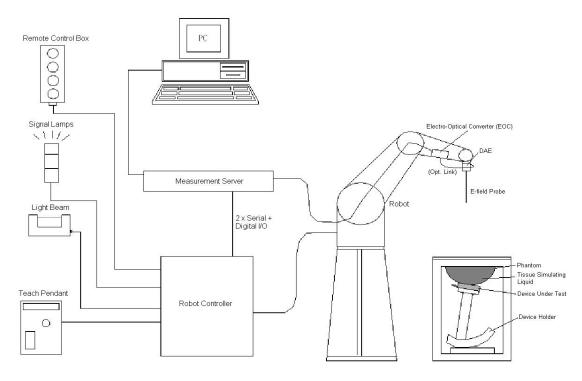
Fig 6.1 SPEAG DASY System Configurations
