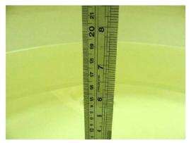
Fig 7.1 Photo of Liquid Height for Head SAR
