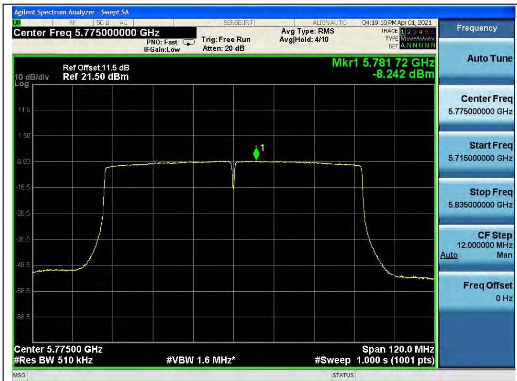
(Channel 155, 5775MHz, 802.11ac (VHT80), ANT0)
