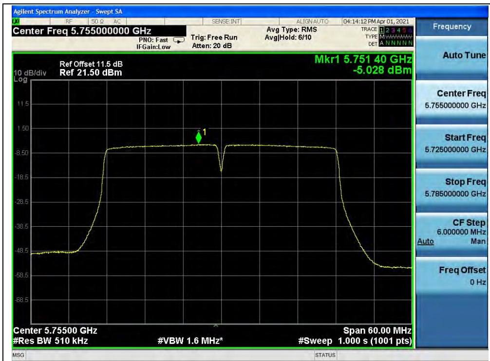
(Channel 151, 5755MHz, 802.11ac (VHT40), ANT0)
