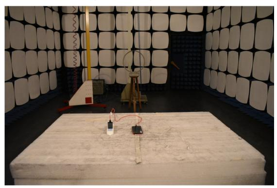
3. Radiated emission (9KHz-30MHz)
