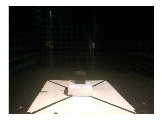
FCC Part15C Radiated Emission above 18-25GHz
