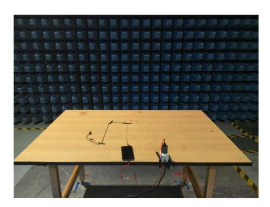
FCC Part15C Radiated Emission above 1-18GHz
